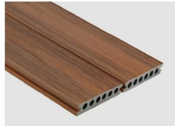
PPD04 Size: 138x22.5 mm Joist span: 350 mm Application: Residential use
