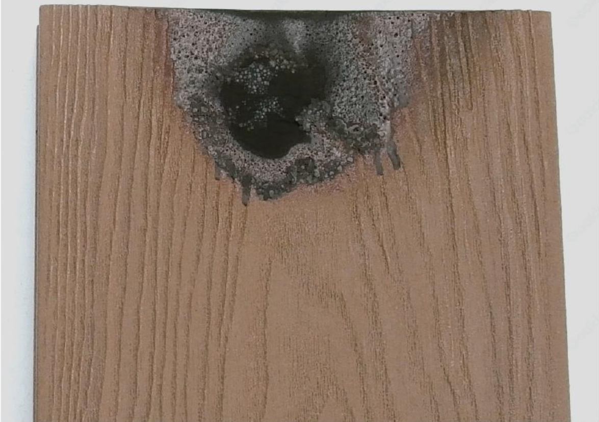
▼ Matshield decking self-extinguishes flame within 2 seconds.
