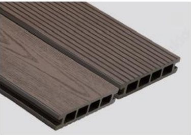
IPD05 Size: 140x25 mm Joist span: 300 mm Application: Residential use
