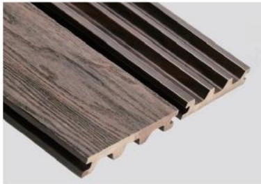
IPD85 Size: 140x23 mm Joist span: 350 mm Application: Commercial use
