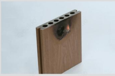
▼ Flame out after ignition source removal.
