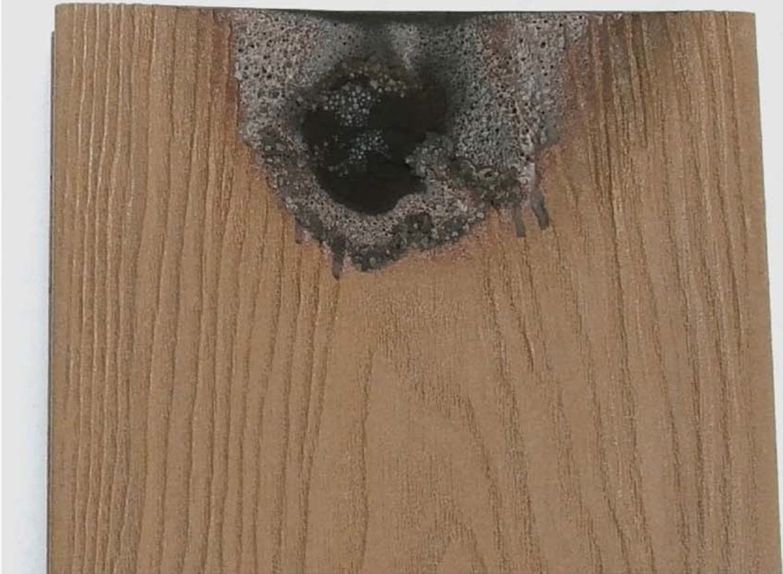
▼ Matshield decking self-extinguishes flame within 2 seconds.
