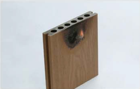
▼ Flame out after ignition source removal.
