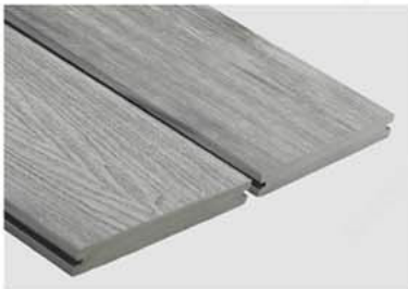
IPD03 Size: 140x20 mm Joist span: 400 mm Application: Commercial use
